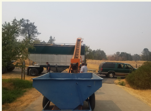
The blue bin is called a hopper and it funnels the almonds onto a conveyor belt which carries them to the top of the trailer and pours them in! Look at all those nuts!
