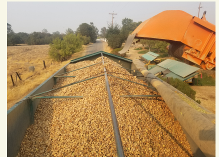
The blue bin is called a hopper and it funnels the almonds onto a conveyor belt which carries them to the top of the trailer and pours them in! Look at all those nuts!
